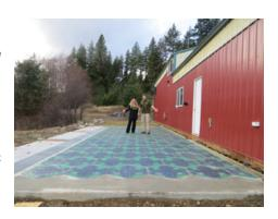
The strong, thick tempered glass has been traction tested, load tested, and impact tested to meet the requirements of roadway conditions. The panels are equipped with a warming element that melts snow and ice in winter months. LED lights can also be incorporated into the panels.
